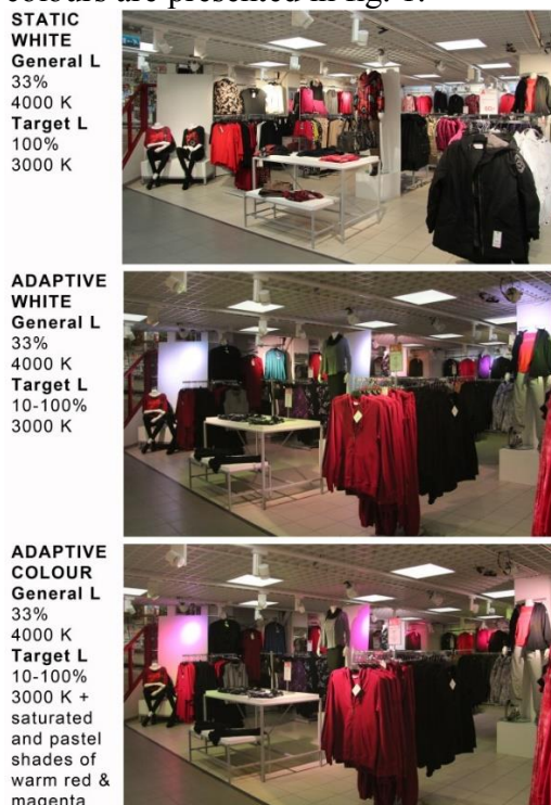
Fig. 1: The tested lighting schemes: Static, Adaptive White and Adaptive Colour.
